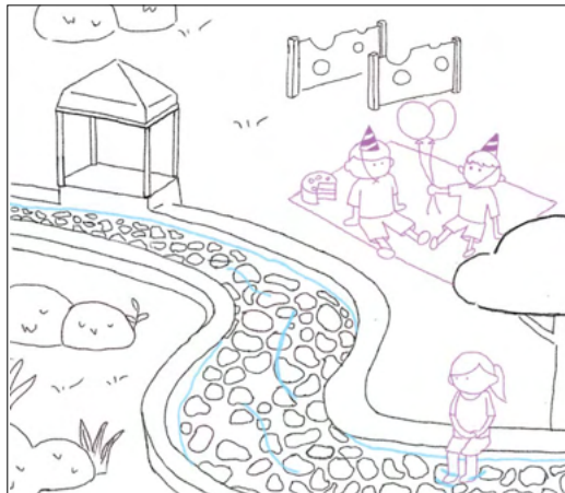
03 Sensory SuDS A multipurpose playgrounds integrated with SuDS that encourage play with water.
